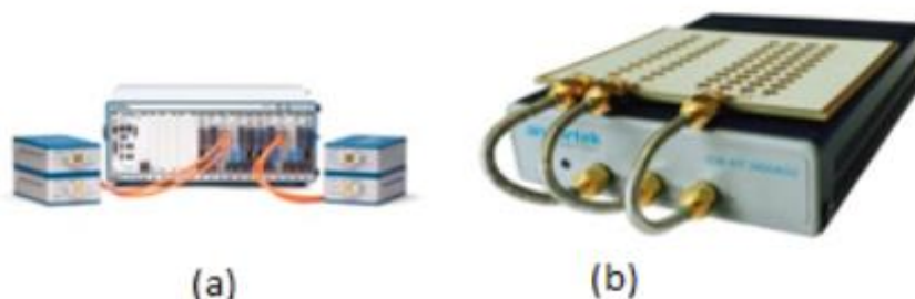
Fig. 6. (a) mmWave Software-Defined Radio (SDR) from NI [63]. (b) mmWave radar kit from Ancortek Source: [64].
