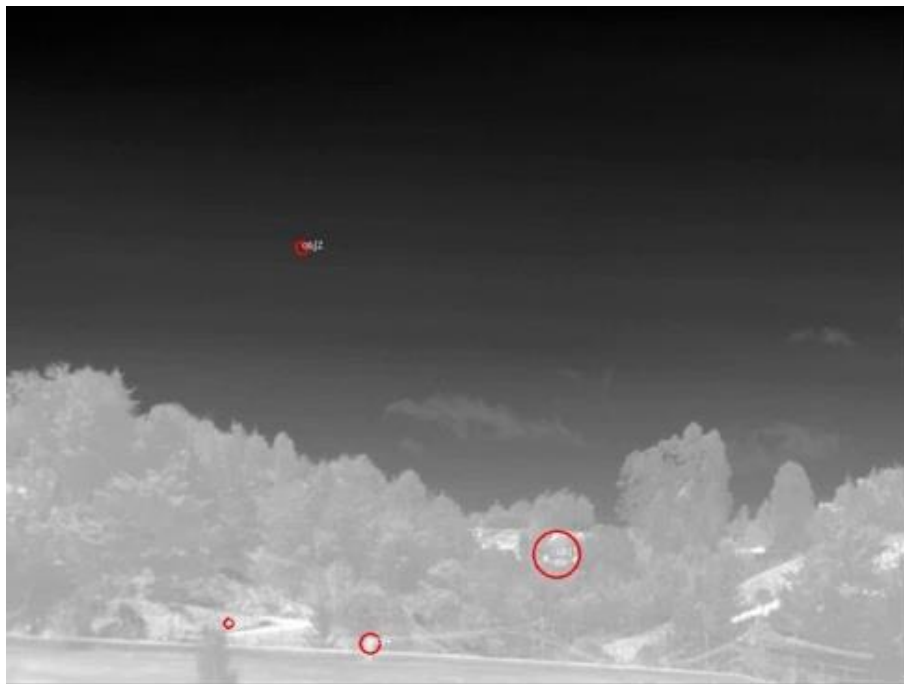
Fig. 5. Thermal object detection; implementation of an algorithm for object detection using a thermal camera. Source: Created by the authors.
