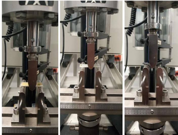
**Figure 4.** Flexure test set-up in kevlar, glassfiber and carbon fiber, respectively
